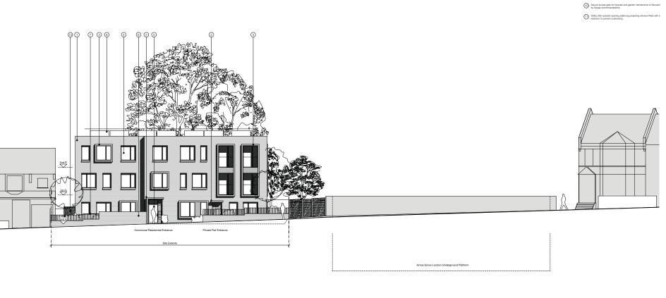
6 Matching brick refuse store enclosure with self-closing painted, galvanised steel gates in RAL 8019.
