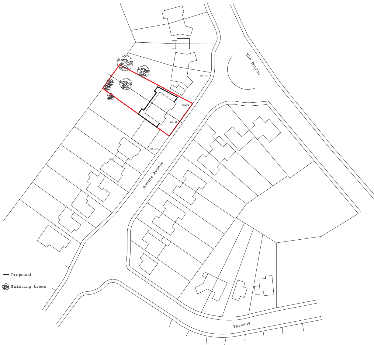
Proposed Block Plan Scale 1/500
