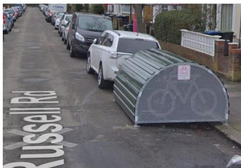
The two hangars retained near driveways will be offset a typical length of 0.8m from the flush kerbs; the same offset relating to parking bays is only 0.3m. Hence the hangars pose no more hindrance to driveway access at the crossovers in question than parked cars do elsewhere.
