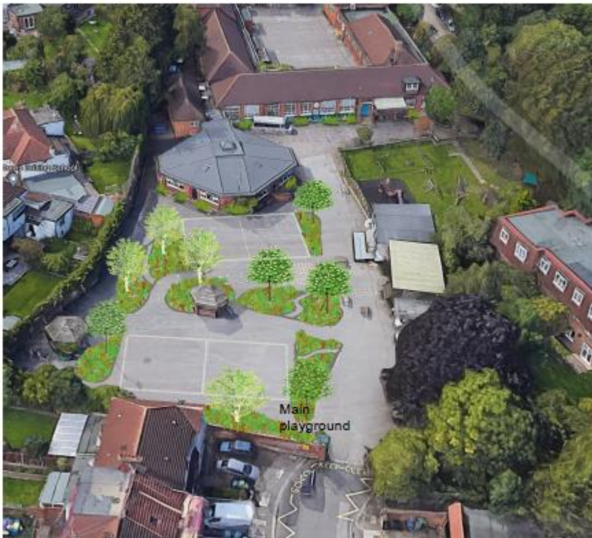
Break up large playground with SuDS features to make a main feature
